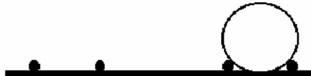
Now remove the barrel and lash the last two spars to the frame (by then you have made 8 square-lashings). Now you're almost done.
